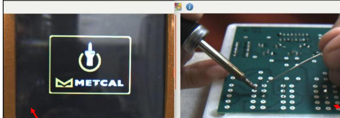
**Process control:** after applying solder, operator will wait until LED result indicated before starting the next joint.
