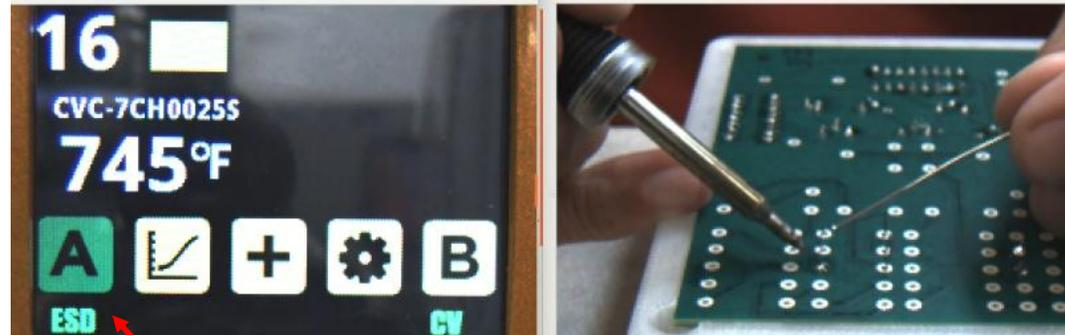
**After applying solder, operator will wait until LED result indicated before starting the next joint.**
