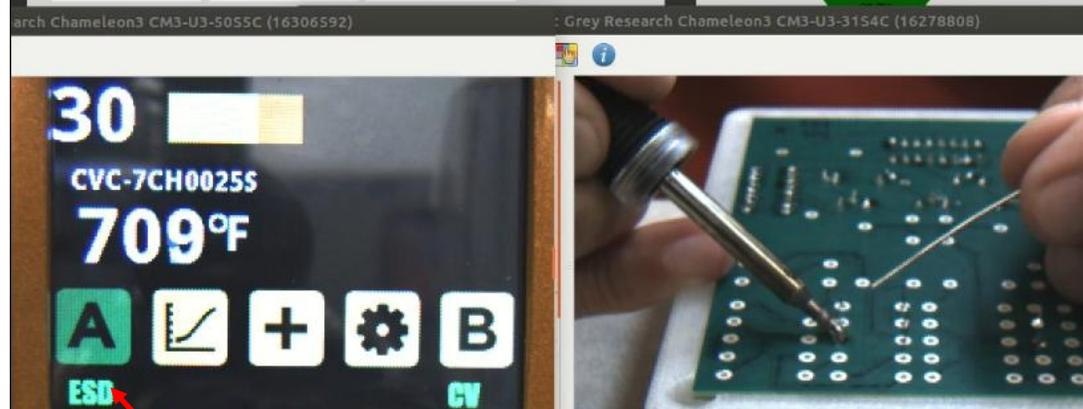
After applying solder, operator will wait until LED result indicated before starting the next joint.
